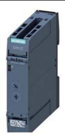
TIMING RELAY, ELECTRONIC, OFF-DELAY, WITHOUT CONTROL SIGNAL OR NON-VOLATILE RELAY DEFINITE PASSING MAKE CONTACT, 7 T. SET. RANGES 0.05S...600S, 24 V AC/DC, 2 CO CONTACTS W. LED, SPRING-TYPE (PUSH-IN) TERMINAL
