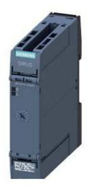
TIME RELAY, ELECTRONIC, WITH STAR-DELTA FUNCTION, 1 CONTACTOR DELAYED, 1 CONTACTOR NON-DELAYED, 1 TIME SET. RANGE 1...20S, 200...240V AC AND 380...440V AC LED, SPRING-LOADED TERMINAL (PUSH-IN)
