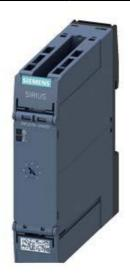
TIME RELAY, ELECTRONIC, WITH STAR-DELTA FUNCTION, 1 CONTACTOR DELAYED, 1 CONTACTOR NON-DELAYED, 1 TIME SET. RANGE 3...60S, 12...240V AC/DC AT AC 50/60HZ, LED, SPRING-LOADED TERMINAL (PUSH-IN)
