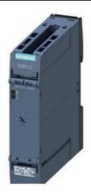
TIME RELAY, ELECTRONIC, WITH STAR-DELTA FUNCTION, 1 CONTACTOR DELAYED, 1 CONTACTOR NON-DELAYED, 1 TIME SET. RANGE 3...60S, 200...240V AC AND 380...440V AC, LED, SPRING-LOADED TERMINAL (PUSH-IN)
