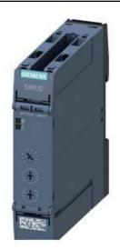
TIME RELAY, MULTI-FUNCTION, 2 CO CONTACTS, 27 FUNCTIONS, 15 TIME SETTING RANGE(1,3,10, 30, 100) (S, MIN, HR), AC/DC 12... 240V, AT AC 50/60HZ, LED, SCREW TERMINAL
