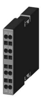
LATERAL AUX.SWITCH BLOCK,SIDE, 2NO, CURR.PATH: 1NO, 1NO, FOR MOTOR CONTACTORS, SZ S0, SPRING-LOADED TERMINAL R: 33/34, 43/44 L: 53/54, 63/64
