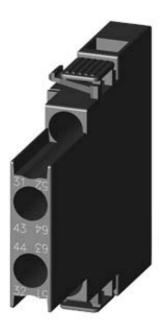
LATERAL AUX.SWITCH BLOCK,SIDE, 1NO+1NC, CURR.PATH: 1NC, 1NO, FOR MOTOR CONTACTORS, SZ S0, SCREW TERMINAL R: 31/32, 43/44 L: 51/52, 63/64
