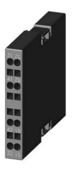
LATERAL AUX.SWITCH BLOCK,SIDE, 2NC, CURR.PATH: 1NC, 1NC, FOR MOTOR CONTACTORS, SZ S0, SPRING-LOADED TERMINAL R: 31/32, 41/42 L: 51/52, 61/62
