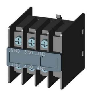
AUX.SWITCH BLOCK,FRONT,3NO, CURR.PATH: 1NO, 1NO, 1NO, F. CONT. RELAYS A. MOTOR CONT., SZ S00 AND S0, RING CABLE LUG CONNECTION .3 / .4,.3 / .4,.3 / .4
