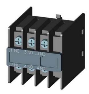
AUX.SWITCH BLOCK,FRONT,2NO+1NC, CURR.PATH: 1NC, 1NO, 1NO, F. CONT. RELAYS A. MOTOR CONT., SZ S00 AND S0, RING CABLE LUG CONNECTION .1 / .2,.3 / .4,.3 / .4
