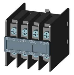
AUX.SWITCH BLOCK, FRONT, 4NO, CURR.PATH: 1NO, 1NO, 1NO, 1NO, FOR CONTACTOR RELAYS, SZ S00, RING CABLE LUG CONNECTION 53 / 54,63 / 64,73 / 74,83 / 84
