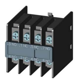
AUX.SWITCH BL 11U,2NO+2NC,FRONT CURR.PATH: 1NO, 1NC, 1NC, 1NO, F. CONT. RELAYS A. MOTOR CONT., SZ S00 AND S0, RING CABLE LUG CONNECTION .3 / .4,.1 / .2,.5 /.6,.7 / .8
