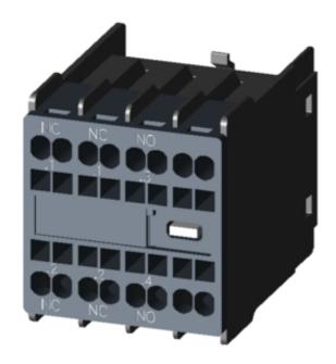
AUX.SWITCH BLOCK,FRONT,1NO+2NC, CURR.PATH: 1NC, 1NC, 1NO, F. CONT. RELAYS A. MOTOR CONT., SZ S00 AND S0, SPRING-LOADED TERMINAL .1 / .2, .1 / .2, .3 / .4
