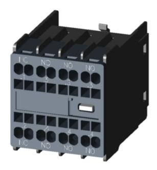
AUX.SWITCH BLOCK,FRONT,3NO+1NC, CURR.PATH: 1NC, 1NO, 1NO, 1NO, F. CONT. RELAYS A. MOTOR CONT., SZ S00 AND S0, SPRING-LOADED TERMINAL .1 / .2,.3 / .4,.3 / .4,.3 / .4
