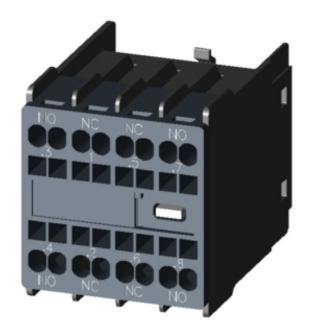
AUX.SWITCH BL 11U,2NO+2NC,FRONT CURR.PATH: 1NO, 1NC, 1NC, 1NO, F. CONT. RELAYS A. MOTOR CONT., SZ S00 AND S0, SPRING-LOADED TERMINAL .3 / .4,.1 / .2,.5 /.6,.7 / .8
