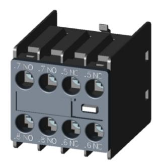
AUX.SWITCH BL 22U,2NO+2NC,FRONT CURR.PATH: 1NO, 1NO, 1NC, 1NC, F. CONT. RELAYS A. MOTOR CONT., SZ S00 AND S0, SCREW TERMINAL .7 / .8,.7 / .8,.5 / .6,.5 / .6
