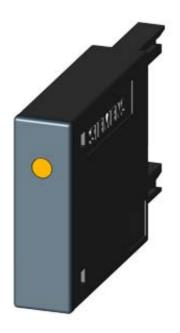
SURGE SUPPRESSOR, SUPPRESSION DIODE WITH LED, DC 150...250V, F. CONT. RELAYS A. MOTOR CONT. SZ S00,
