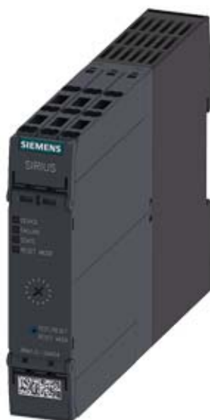
MOTOR STARTER SIRIUS 3RM1 DIRECT STARTER 500 V; 1,6-7,0 A; 24 V DC PUSH-IN CONNECTION SYSTEM
