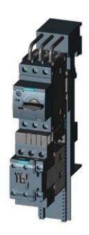
LOAD FEEDER FUSELESS DIRECT START, AC 400V, SZ. S0, 27...32A, AC 230V SCREW CONNECTION FOR BUSBAR SYSTEMS 60MM TYPE OF COORD. 2,IQ = 150KA (ALSO ACHIEVES TYPE OF COORD.1) 1NO+1NC (CONTACTOR)
