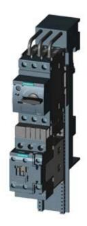
LOAD FEEDER FUSELESS DIRECT START, AC 400V, SZ S0, 11...16A, AC 230V SCREW CONNECTION FOR BUSBAR SYSTEMS 60MM TYPE OF COORDINATION 2, IQ = 150KA (ALSO FULFILLS TYPE OF COORDINATION 1) 1NO+1NC (CONTACTOR)
