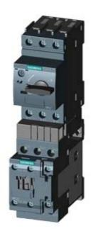
LOAD FEEDER FUSELESS DIRECT START, AC 400V, SZ. S0, 27...32A, AC 230V SCREW CONNECTION FOR RAIL MOUNTING, TYPE OF COORD. 2,IQ = 150KA (ALSO ACHIEVES TYPE OF COORD.1) 1NO+1NC (CONTACTOR)
