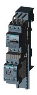
LOAD FEEDER FUSELESS DIRECT START, AC 400V, SZ S0, 14. . .20A, DC 24V SCREW TERMINAL FOR BUSBAR SYSTEMS 60MM, TYPE OF COORDINATION 1, IQ = 150KA 1NO+1NC (CONTACTOR)
