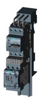
LOAD FEEDER FUSELESS DIRECT START, AC 400V, SZ. S0, 9. . .12.5A, DC 24V SCREW CONNECTION FOR BUSBAR SYSTEMS 60MM TYPE OF COORD. 2,IQ = 150KA (ALSO ACHIEVES TYPE OF COORD.1) 1NO+1NC (CONTACTOR)
