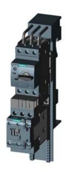
LOAD FEEDER FUSELESS DIRECT START, AC 400V, SZ S0, 3.5...5A, DC 24V SCREW CONNECTION FOR BUSBAR SYSTEMS 60MM TYPE OF COORDINATION 2, IQ = 150KA (ALSO FULFILLS TYPE OF COORDINATION 1) 1NO+1NC (CONTACTOR)
