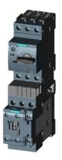
LOAD FEEDER FUSELESS DIRECT START, AC 400V, SZ S0, 14. . .20A, DC 24V SCREW TERMINAL FOR RAIL-MOUNTING, TYPE OF COORDINATION 1, IQ = 150KA 1NO+1NC (CONTACTOR)
