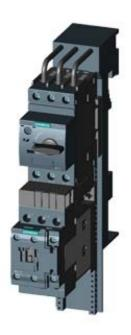
LOAD FEEDER FUSELESS DIRECT START, AC 400V, SZ. S0, 7...10A, DC 24V SCREW CONNECTION FOR BUSBAR SYSTEMS 60MM TYPE OF COORD. 2,IQ = 150KA (ALSO ACHIEVES TYPE OF COORD.1) 1NO+1NC (CONTACTOR)
