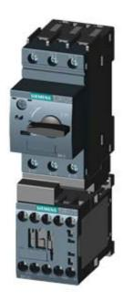
LOAD FEEDER FUSELESS DIRECT START, AC 400V, SZ S00 5,5. . .8A, AC 230V SCREW CONNECTION FOR RAIL-MOUNTING, TYPE OF COORDINATION 1, IQ = 150KA 1NO (CONTACTOR)
