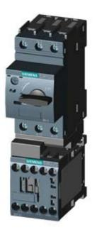
LOAD FEEDER FUSELESS DIRECT START, AC 400V, SZ S00 3.5. . .5A, AC 230V SCREW CONNECTION FOR RAIL-MOUNTING, TYPE OF COORDINATION 1, IQ = 150KA 1NO (CONTACTOR)
