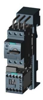
LOAD FEEDER FUSELESS DIRECT START, AC 400V, SZ S00 5,5. . .8A, DC 24V SCREW CONNECTION FOR BUSBAR SYSTEMS 60MM TYPE OF COORDINATION 1, IQ = 150KA 1NO (CONTACTOR)
