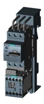
LOAD FEEDER FUSELESS DIRECT START, AC 400V, SZ S00 3.5. . .5A, AC 230V SCREW CONNECTION FOR BUSBAR SYSTEMS 60MM TYPE OF COORDINATION 1, IQ = 150KA 1NO (CONTACTOR)
