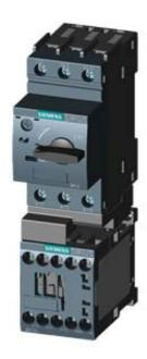
LOAD FEEDER FUSELESS DIRECT START, AC 400V, SZ S00 9. . .12.5A, AC 230V SCREW CONNECTION FOR RAIL-MOUNTING, TYPE OF COORDINATION 1, IQ = 150KA 1NO (CONTACTOR)
