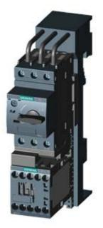
LOAD FEEDER FUSELESS DIRECT START, AC 400V, SZ S00 1.4. . .2A, DC 24V SCREW CONNECTION FOR BUSBAR SYSTEMS 60MM TYPE OF COORDINATION 2, IQ = 150KA (ALSO FULFILLS TYPE OF COORDINATION 1) 1NO (CONTACTOR)
