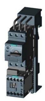
LOAD FEEDER FUSELESS DIRECT START, AC 400V, SZ S00 2.8. . .4A, AC 230V SCREW CONNECTION FOR BUSBAR SYSTEMS 60MM TYPE OF COORDINATION 2, IQ = 150KA (ALSO FULFILLS TYPE OF COORDINATION 1) 1NO (CONTACTOR)
