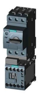
LOAD FEEDER FUSELESS DIRECT START, AC 400V, SZ S00 4.5. . .6.3A, DC 24V SCREW CONNECTION FOR RAIL-MOUNTING, TYPE OF COORDINATION 1, IQ = 150KA 1NO (CONTACTOR)
