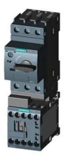
LOAD FEEDER FUSELESS DIRECT START, AC 400V, SZ S00 1.8. . .2.5A, DC 24V SCREW CONNECTION FOR RAIL-MOUNTING, TYPE OF COORDINATION 2, IQ = 150KA (ALSO FULFILLS TYPE OF COORDINATION 1) 1NO (CONTACTOR)
