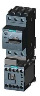
LOAD FEEDER FUSELESS DIRECT START, AC 400V, SZ S00 3.5. . .5A, DC 24V SCREW CONNECTION FOR RAIL-MOUNTING, TYPE OF COORDINATION 1, IQ = 150KA 1NO (CONTACTOR)
