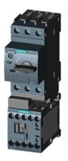
LOAD FEEDER FUSELESS DIRECT START, AC 400V, SZ S00 0.7...1A, AC 230V SCREW CONNECTION FOR RAIL-MOUNTING, TYPE OF COORDINATION 2, IQ = 150KA (ALSO FULFILLS TYPE OF COORDINATION 1) 1NO (CONTACTOR)
