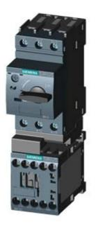
LOAD FEEDER FUSELESS DIRECT START, AC 400V, SZ S00 0.9. . .1.25A, AC 230V SCREW CONNECTION FOR RAIL-MOUNTING, TYPE OF COORDINATION 2, IQ = 150KA (ALSO FULFILLS TYPE OF COORDINATION 1) 1NO (CONTACTOR)
