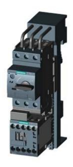
LOAD FEEDER FUSELESS DIRECT START, AC 400V, SZ S00 0.55. . . 0.8A, AC 230V SCREW CONNECTION FOR BUSBAR SYSTEMS 60MM TYPE OF COORDINATION 2, IQ = 150KA (ALSO FULFILLS TYPE OF COORDINATION 1) 1NO (CONTACTOR)
