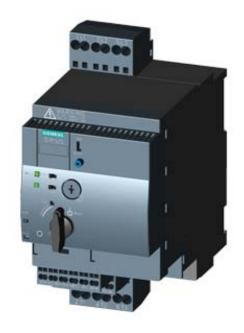
SIRIUS, COMPACT STARTER, REVERSING STARTER 690 V, 24 V AC/DC, 50 ... 60 HZ, 3 ... 12 A, IP20, MAIN CIRCUIT CONNECTION: SPRING-LOADED TERMINAL, AUXILIARY CIRCUIT CONNECTION: SPRING-LOADED TERMINAL
