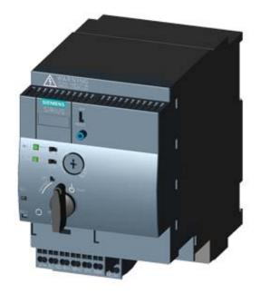
SIRIUS, COMPACT STARTER, REVERSING STARTER 690 V, 110 ... 240 V AC/DC, 50 ... 60 HZ, 0.32 ... 1.25 A, IP20, MAIN CIRCUIT CONNECTION: PLUG-IN, W/O TERMINALS, AUXILIARY CIRCUIT CONNECTION: SPRING-LOADED TERMINAL
