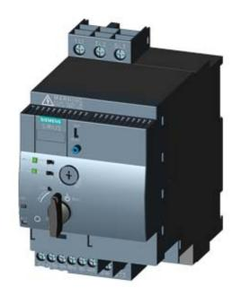
SIRIUS, COMPACT STARTER, REVERSING STARTER 690 V, 24 V AC/DC, 50 ... 60 HZ, 3 ... 12 A, IP20, MAIN CIRCUIT CONNECTION: SCREW TERMINAL, AUXILIARY CIRCUIT CONNECTION: SCREW TERMINAL
