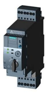
SIRIUS, COMPACT STARTER, DIRECT STARTER 690 V, 24 V AC/DC, 50 ... 60 HZ, 3 ... 12 A, IP20, CONNECTION MAIN CIRCUIT: SPRING-LOADED TERMINAL, CONNECTION AUXILIARY CIRCUIT: PLUGGABLE, WITHOUT TERMINALS
