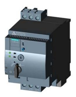
SIRIUS, COMPACT STARTER, REVERSING STARTER 690 V, 24 V AC/DC, 50 ... 60 HZ, 1 ... 4 A, IP20, MAIN CIRCUIT CONNECTION: SCREW TERMINAL, AUXILIARY CIRCUIT CONNECTION: PLUG-IN, W/O TERMINALS
