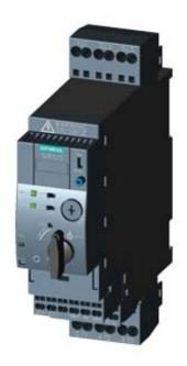
SIRIUS, COMPACT STARTER, DIRECT STARTER 690 V, 110 ... 240 V AC/DC, 50 ... 60 HZ, 0.1 ... 0.4 A, IP20, CONNECTION MAIN CIRCUIT: SPRING-LOADED TERMINAL,
