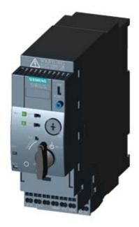
SIRIUS, COMPACT STARTER, DIRECT STARTER 690 V, 24 V AC/DC, 50 ... 60 HZ, 1 ... 4 A, IP20, CONNECTION MAIN CIRCUIT: PLUGGABLE, WITHOUT TERMINALS, CONNECTION AUXILIARY CIRCUIT: SPRING-LOADED TERMINAL
