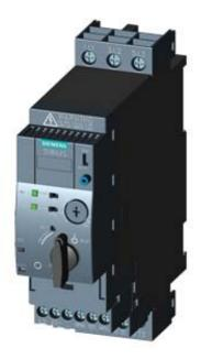
SIRIUS, COMPACT STARTER, DIRECT STARTER 690 V, 24 V AC/DC, 50 ... 60 HZ, 3 ... 12 A, IP20, CONNECTION MAIN CIRCUIT: SCREW TERMINAL, CONNECTION AUXILIARY CIRCUIT: SCREW TERMINAL
