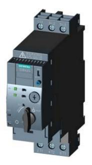
SIRIUS, COMPACT STARTER, DIRECT STARTER 400 V, 24 V AC/DC, 50 ... 60 HZ, 8 ... 32 A, IP20, CONNECTION MAIN CIRCUIT: SCREW TERMINAL, CONNECTION AUXILIARY CIRCUIT: PLUGGABLE, WITHOUT TERMINALS
