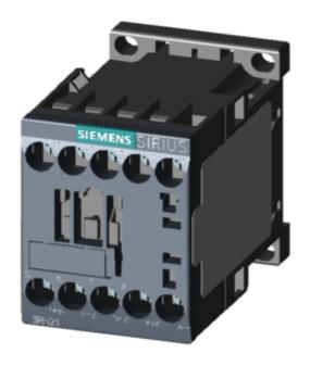
COUPLING CONTACTOR RELAY, 3NO+1NC, DC 110V, 0.7..1.25\*US, W/ INTEGRATED SUPPRESSOR DIODE, SIZE S00, SCREW TERMINAL
