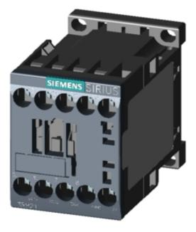
CONTACTOR RELAY, 2NO+2NC, DC 24V, W/ INTEGRATED DIODE, SIZE S00, SCREW TERMINAL
